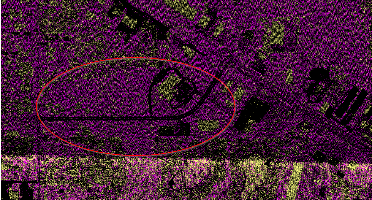
Figure 3. Example of an area showing low near infrared reflectivity from fresh asphalt and roof tops
