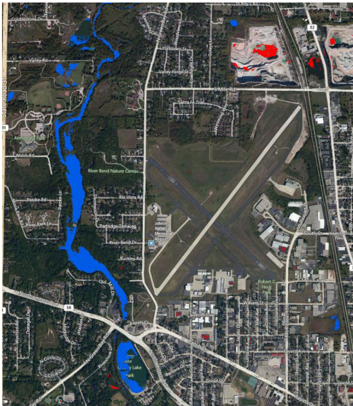
Figure 5: Example of Legitimate Data Voids Blue Areas represent Water Bodies and Red Areas are NIR Reflectivity
