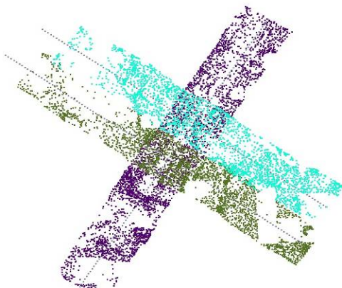
Figure 2: Tie plane depiction of calibration
