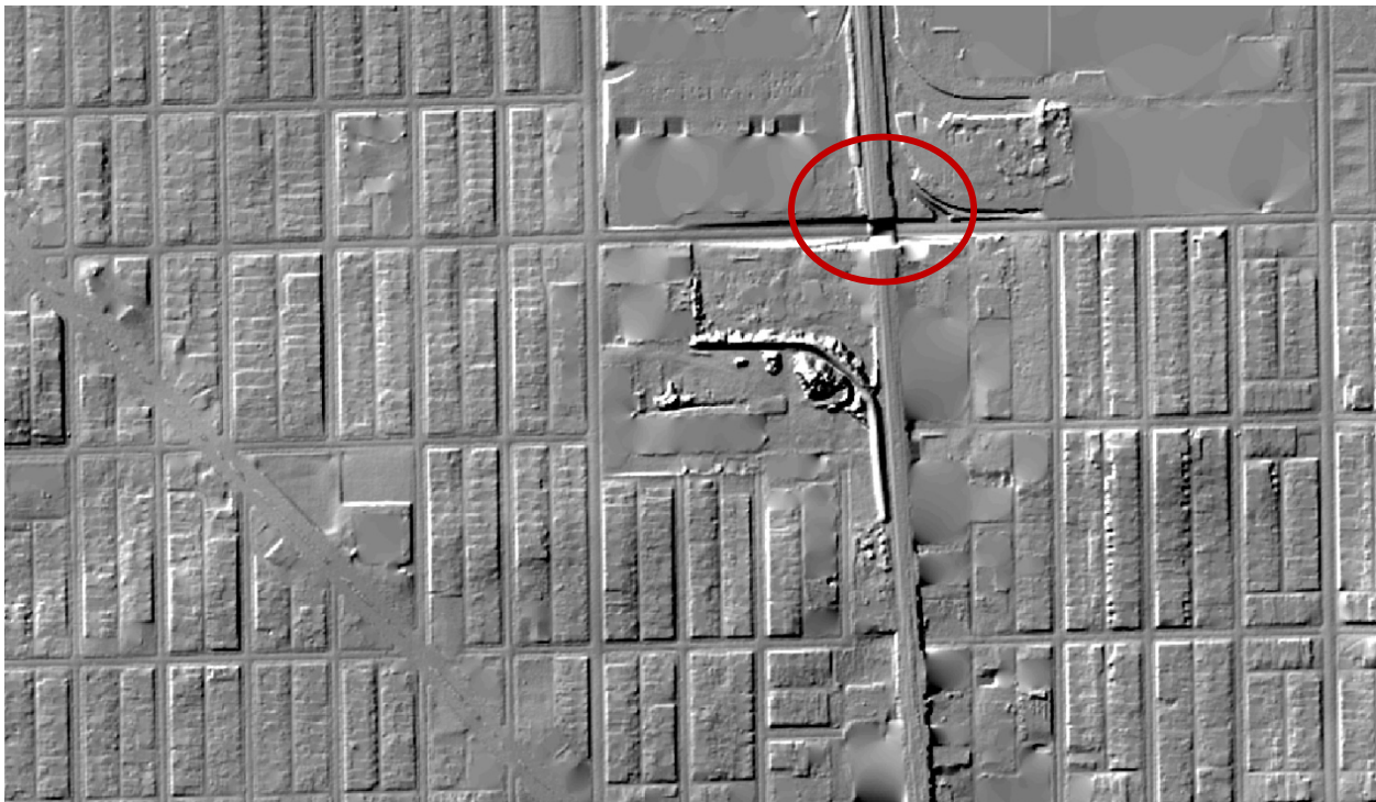
Figure 8 shows an example of the Hillshade displayed at 1:4000 scale. The hillshade was used to confirm edge consistency and to look for artifacts and systematic errors in the data. The area within the red circle shows proper removal of ground points from an overpass.
