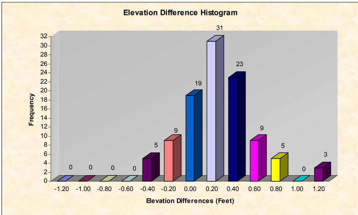
**Figure 4 – Histogram of Elevation Discrepancies within 0.2 ft bands**
