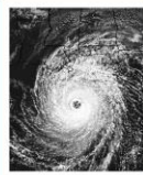
Above: Simulated image of ABI Band 1 for Hurricane Katrina. This image was simulated via measurements of high spatial resolution central model runs and advanced central model radiative transfer models. (Credit: CIMSS)
