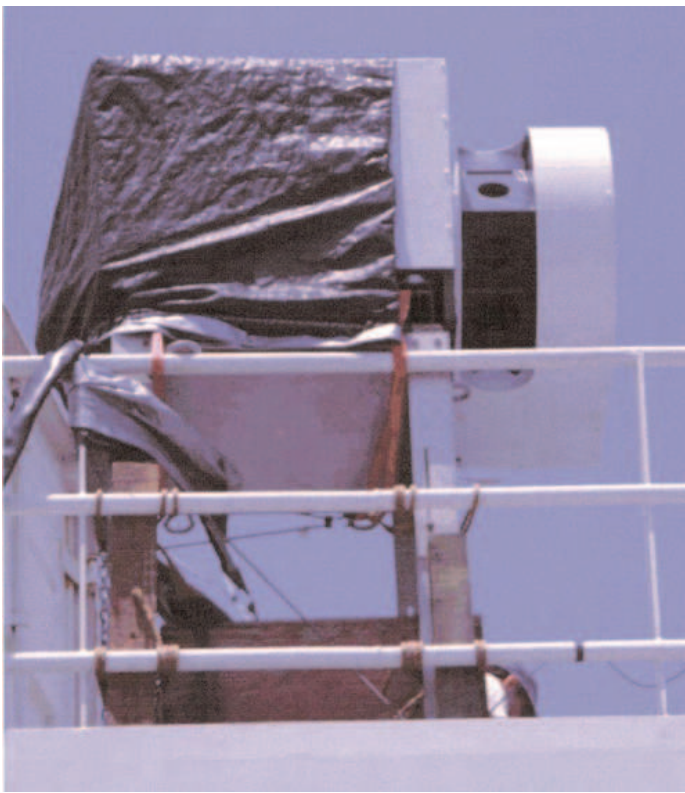
Figure 2.9 The M-AERI installed on the NOAAS Ronald H. Brown. The instrument is on the forward 02 deck at the starboard railing. The field of view intersects the sea surface ahead of the bow wave.
