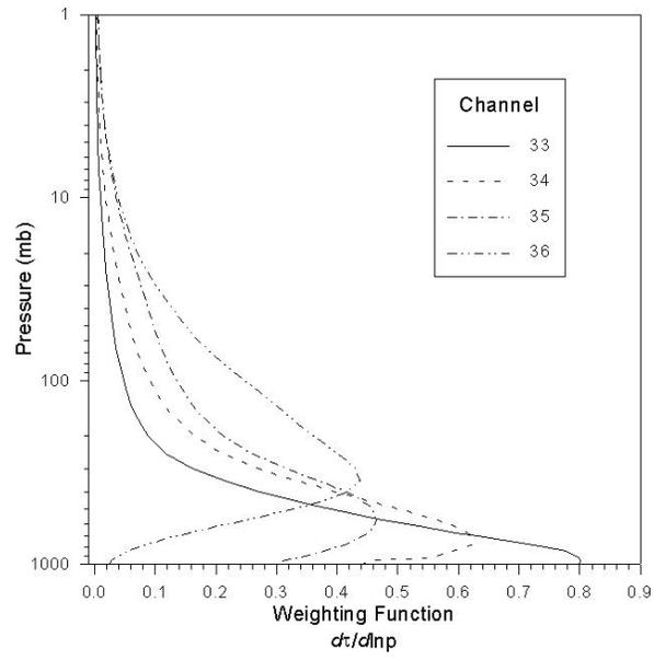
**Figure 4. Weighting functions for the four MODIS channels in the CO<sub>2</sub> absorption band**
