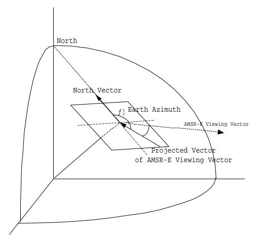
Figure 1: NASDA definition of Earth Azimuth
