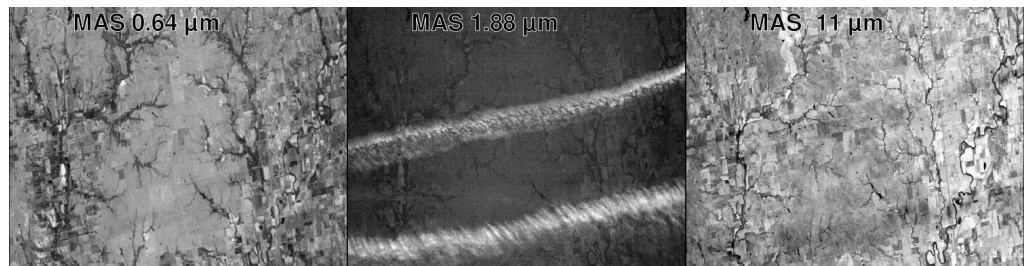
NASA's MODIS Airborne Simulator (MAS) was used, in part, to demonstrate several of the spectral bands of the ABI. In this case from the MAS, upper-level cirrus are clearly evident in the 1.88 μm image (center panel), but much less in the traditional visible band (left) and the longwave window band (right). Credit: NASA and SSEC
