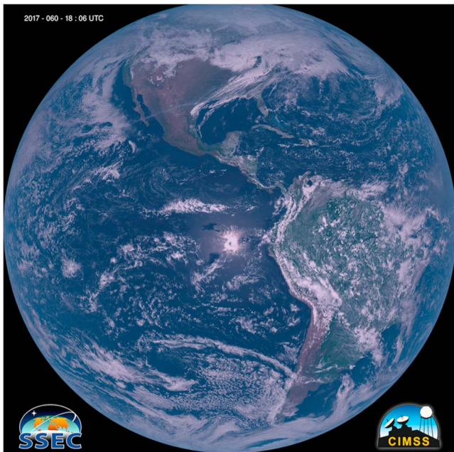
Figure 6. GOES-16 true color (natural) Red-Green-Blue image for 1 March 2017, at 18:06 UTC. The green band in this case was generated using the weighted nudging approach with an inverse hyperbolic sine function enhancement applied.
