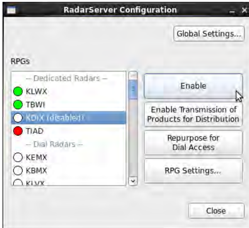
Exhibit 7.8-6. The connection has been disabled, but is still listed as a dedicated radar
