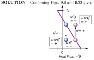
Both the up-moving and down-moving portions of a turbulent eddy contribute to positive  $w'w'\theta'$ . Thus the average of both up and down gives  $\overline{w'w'\theta'} = \text{positive}$ . This generic method can be used with many other turbulent terms, but give a reasonable estimate only if no large eddies are present.
