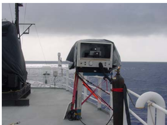
Figure 1: The Marine Atmospheric Emitted Radiance Interferometer located onboard the NOAA Ship Ronald H. Brown during the 2004 Aerosol and Ocean Science Expedition (AEROSE-I).
